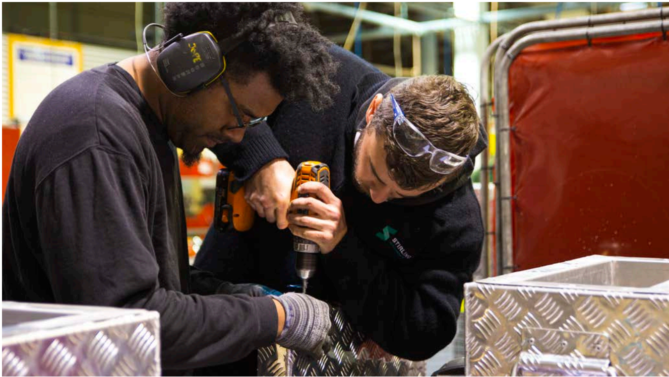
Engineering students fabricating custom-made cooling boxes as a part of a class project.
